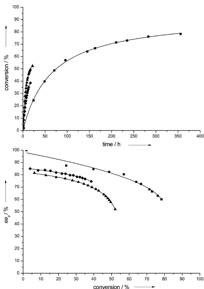
**Figure 1.** Enzymatic kinetic resolution of 3-hydroxy octanoic acid methyl ester by Novozym 435 and vinyl acetate in hexane containing different amounts of Et<sub>3</sub>N. Plots of a) conversion versus time and b) enantiomeric excess versus conversion; ■ = reaction without Et<sub>3</sub>N, ◆ = reaction with catalytic amount Et<sub>3</sub>N, ▲ = Et<sub>3</sub>N as a co-solvent.
