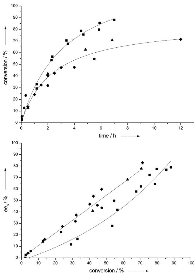
**Figure 2.** Hydrolysis of 3-hydroxy fatty acid esters **2** (●), **3** (▲), **4** (◆), and **5** (■) by Novozym 435 dissolved in Et<sub>3</sub>N; a) reaction rate; b) plot enantiomeric excess versus conversion.
