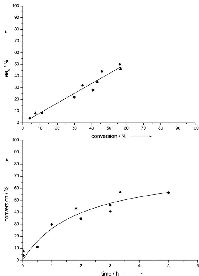
**Figure 3.** Hydrolysis of 3-hydroxy fatty acid esters **2** (●), **3** (▲), and **4** (◆) by Novozym 435 dissolved in a 2% DABCO solution in hexane; a) reaction rate; b) enantiomeric excess versus conversion.
